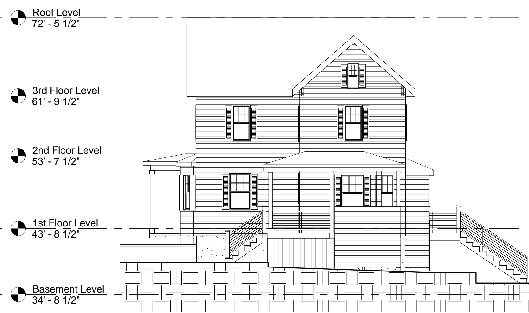
6 Existing North Elevation 1/8" = 1'-0"
